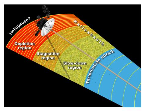
Fig. 3-3. Voyagers 1 and 2 exploration of the outer regions of the solar bubble as of 2013.
