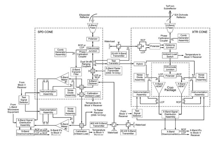
Fig. 3-7. DSS-14 and DSS-43 microwave and transmitter block diagram.
