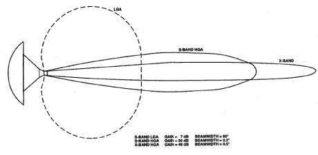
Fig. 3-6. Voyager SXA patterns and beamwidths.
