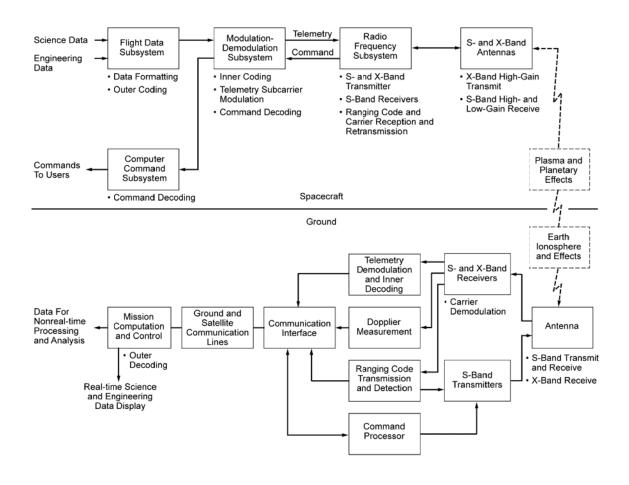
Fig. 3-4. Overview of spacecraft and ground telecommunications functions for Voyager.
