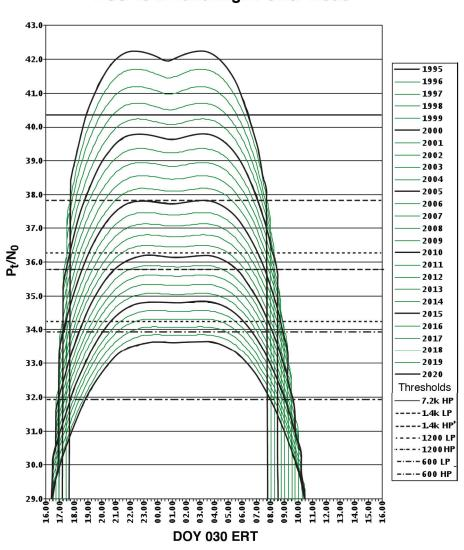
VGR-2 Annual P<sub>t</sub>/N<sub>0</sub> Profiles DSS-43 X-Band High Power Mode
