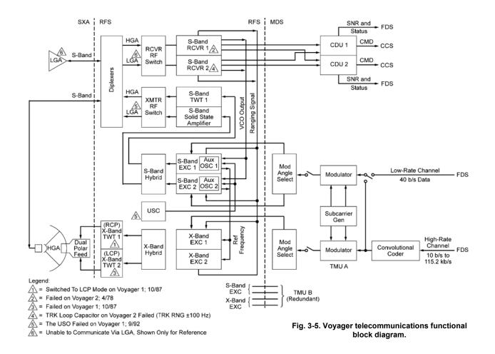
working as a redundant pair. Microwave components provide radio frequency (RF) filtering and switching for connecting the transmitters and receivers to the high-gain or low-gain antenna.
